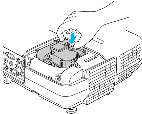
9. Once the lamp is fully inserted, tighten its screws.
