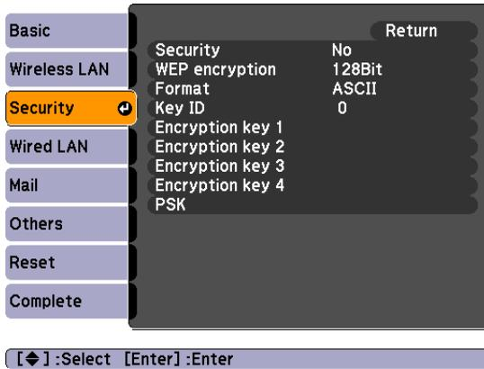
4. For the WEP encryption setting, select **128Bit** or **64Bit** and press **Enter**.
