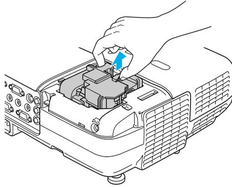
7. Gently insert the new lamp. (If it doesn't fit easily, make sure it is facing the right way.)
