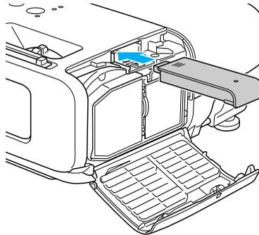
3. Fasten the module using the screw that came with it.
