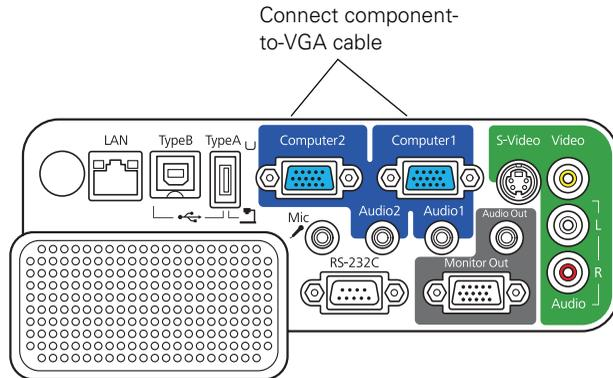
2. Insert the three component ends of the component-to-VGA cable into the color-coded output ports on your video source, usually labelled Y, Pb, Pr or Y, Cb, Cr.
