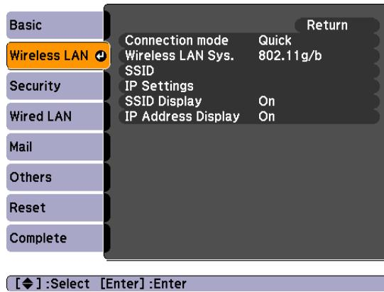
4. Make sure **Quick** is selected for the **Connection mode**. If not, use the
