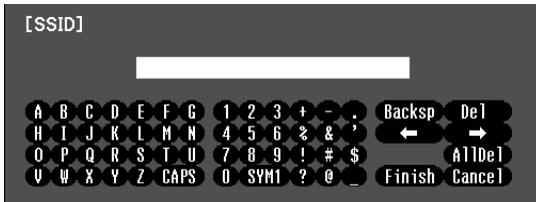
Note that the SSID is case-sensitive (if you enter the name in uppercase on the projector, you must type it the same way on the computer connecting to the projector).
