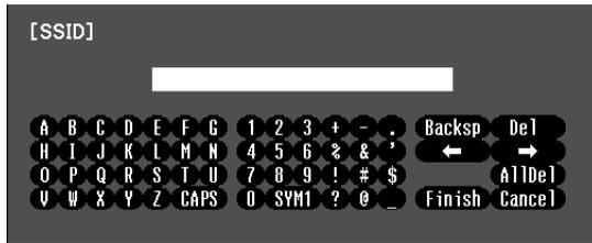
Note that the SSID is case-sensitive (if you enter the name in uppercase on the projector, you must type it the same way on the computer connecting to the projector).
