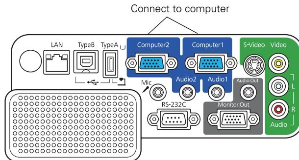
2. You can connect an optional stereo mini-jack audio cable to play sound through the projector (see page 49), or connect the USB cable to use the remote control as a mouse (see page 42).
