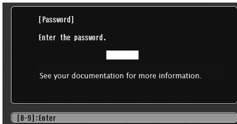
Hold down the **Num** button on the remote control and use the numeric keypad to enter the four digit password.
