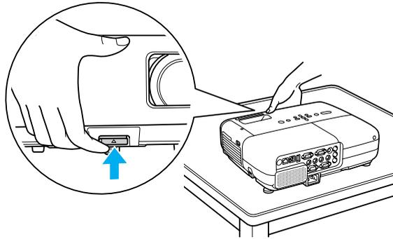
2. Once the image is positioned where you want it, release the lever to lock the foot in position.
