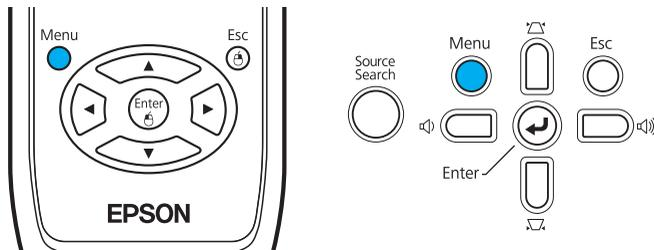
From the Settings menu, select **Keystone** and press **Enter**. Use the
