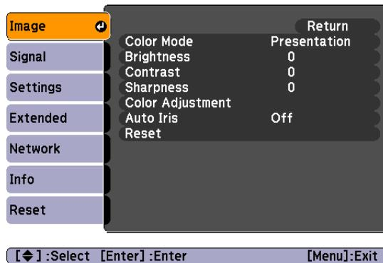
2. Use the
