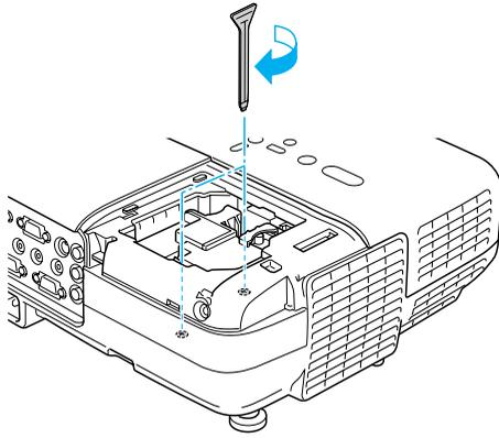
10. Replace the lamp cover, then tighten its screw.
