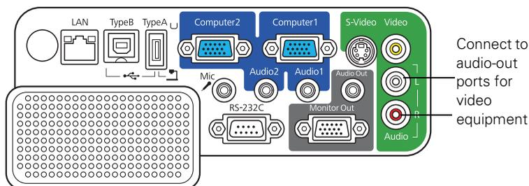
2. Connect the red and white plugs on the other end to the corresponding color-coded audio output jacks on your video source.
