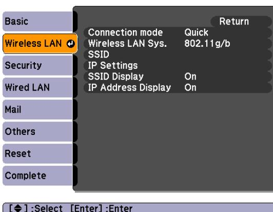
4. Make sure **Advanced** is selected for the Connection mode. If not, use the
