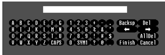
6. If you want to create a password for using PLink to control the projector, highlight **PLink Password**, press **Enter**, and enter a password of up to 8 alphanumeric characters. When you're done, highlight **Finish** and press **Enter**.
