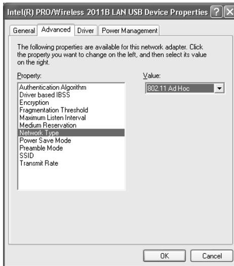
5. Check your wireless card or adapter device settings. (Depending on the type of card or adapter you're using, some of the settings may be different than those listed here.)
