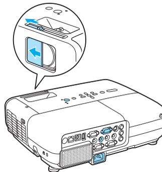
2. Plug one end of the power cable into the projector, and the other end into an electrical outlet.
