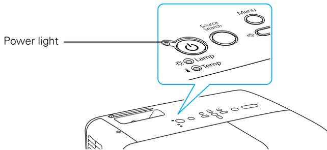
3. Press the
