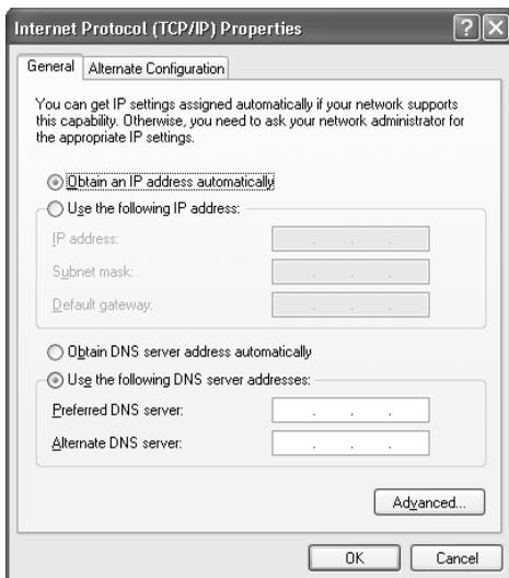
10. If your access point uses DHCP, select **Obtain an IP address automatically**. Otherwise select **Use the following IP address** and enter the required information:
